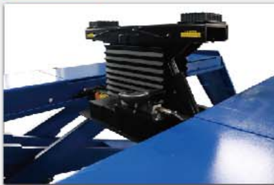
Rolling jack RJ7000Y (Capacity 3200kg)
