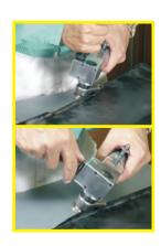
Forged and hardened steel de-crimping head is specially designed to unfold the steel flanges of a damaged door skin with a minimum of physical effort.
