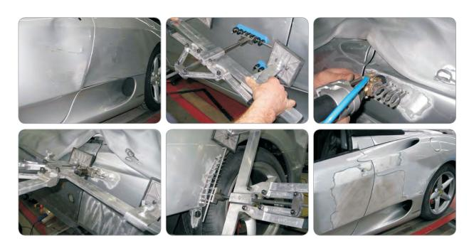
The repair of the side panel and door on this Ferrari 360 spider poses a real challenge for every panel repairer. Knowing the problems of panel part replacements, the car owner absolutely wanted to avoid the common exchange of door and side panel on this convertible car. The door alone has an extremely long delivery time and costs more than Rs 1,75,000. When the owner checked the car before the paint job, he was enthusiastic and was impressed with the high quality of the repair.
