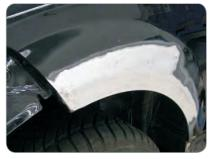
A damage like this cannot be repaired at all using conventional methods. After the preliminary dressing with gluing technology AluBits are being welded along the deformation with the special welding gun. Then the Strong-Puller is being used to finish the repair in a controlled way. The achievable time savings compared to part replacement amount to over sixty percent.
